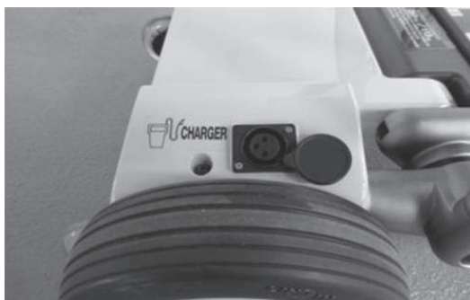
battery charging Port
